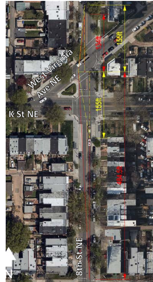
Diagram showing limited SSD for southbound vehicles on 8 th Street NE
