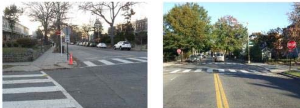
Left: 10 th Street lacks back-to-back stop-control sign panels. Right: Back-to-back sign panels at 9 th Street.
